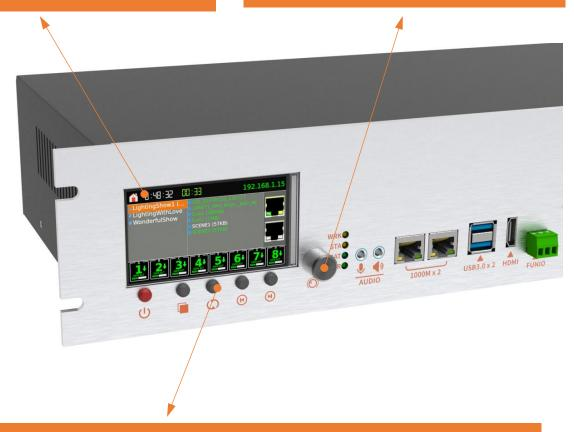
The operation keys, from left to right are Power key, Switch key, Focus key, Left key and Right key.
